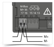
Fig.: M-Bus interface with 2-pole plug contact
