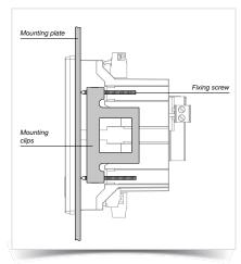
Fig.: The fastening into a switchboard is implemented via the side-mounted fastening clamps (UMG 96RM-P / UMG 96RM-CBM)
