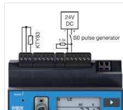
Fig.: Example temperature input (KTY83) and S0 pulse transducer
